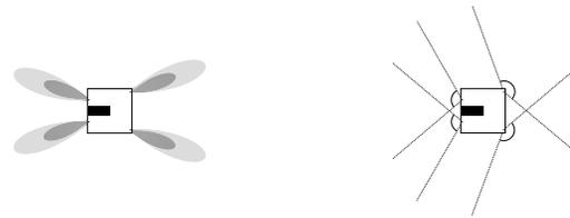
Figure 3: **Left:** The extent to which reflected IR can be sensed (dark grey area), and the extent to which IR beam is perceptible to other robots (light grey area). **Right:** The angles from which a robot can perceive the IR emissions of others
