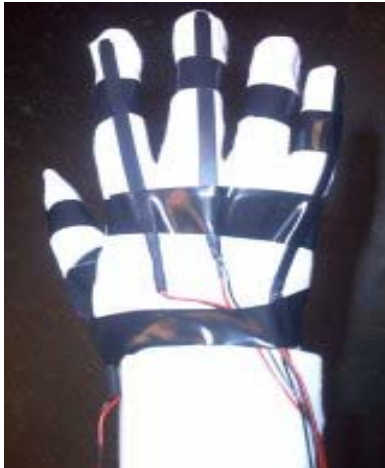
Figure 1. Flex sensors location on the fingers.
